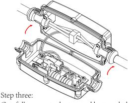
Carefully separate the top and bottom halves of the Power Watchdog Unit.
