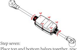
Place top and bottom halves together, rescrew all the screws, tighten down the cable gland connectors.
