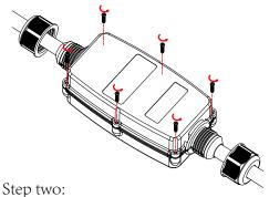
Unscrew the 8 Phillips screws (M3\*16) on the back side of the unit.
