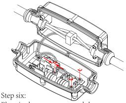
Place in the new surge module, rescrew the 3 screws, clip together the wire connections.
