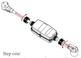
Loosen and unscrew the top and bottom cable gland connectors.
