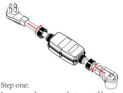
Loosen and unscrew the top and bottom cable gland connectors.
