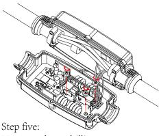
Unscrew the 3 phillips screws. Holding down the surge board.
