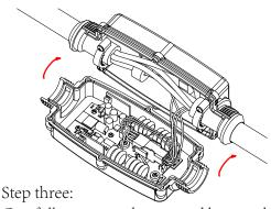
Carefully separate the top and bottom halves of the Power Watchdog Unit.
