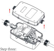
Carefully separate the top and bottom halves of the Power Watchdog Unit.
