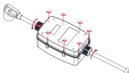
Step seven: Place top and bottom halves together, rescrew all the screws, tighten down the cable gland connectors. \*Do not overtighten the screws.
