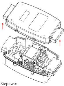
Carefully separate the top and bottom halves of the Power Watchdog Unit.
