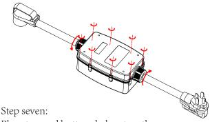
Place top and bottom halves together, rescrew all the screws, tighten down the cable gland connectors.
