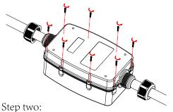
Unscrew the 8 Phillips screws (M3\*16) on the back side of the unit.
