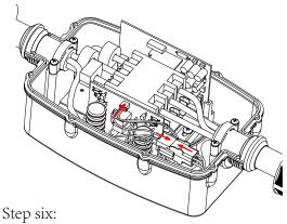
Slide in the new surge module into the slots inside the Power Watchdog unit. clip together the connections.
