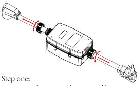
Loosen and unscrew the top and bottom cable gland connectors.
