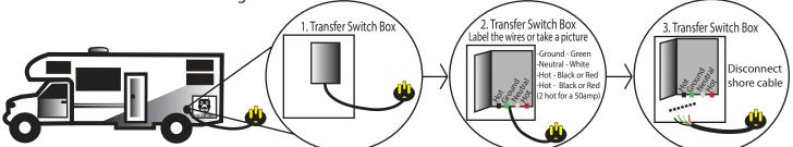
Step 3: Use the supplied male "plug/cord" in the kit and wire it into your transfer switch or main breaker.
