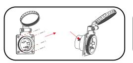
Turn off Rv's main breaker. Use a screwdriver to loosen and remove the four screws and pull out the old inlet out of the RV. Loosen screws and disconnect the old inlet to any wires.
