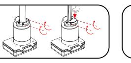
Tighten the screws on the strain relief clamp until they are snug around the cable. You may need to use the optional bushing to have a proper snug fit. (4.5-5.5 ln/Lb).
