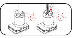
Tighten the screws on the strain relief clamp until they are snug around the cable. You may need to use the optional bushing to have a proper snug fit. (4.5-5.5 ln/Lb).
