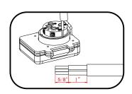
Please strip the wires as shown; strip off 1 5/8" of the outer insulation layer of the cable, and only 5/8" of the colored insulation of the conductor cables. Make sure the wire condition is good, full strands and shiny copper.
