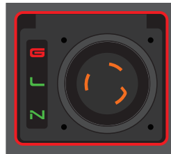
Missing Ground G - Red L, N - Green Border - Flashing Red
