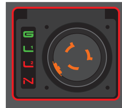
Line 2 and Neutral Reversed L2 and N - Red G, L1 - Green Border - Flashing Red
