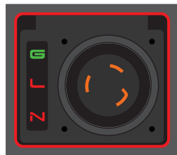
Line and Neutral Reversed L, N - Red G - Green Border - Flashing Red
