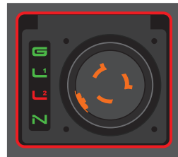
Missing Line 2 L2 - Red G, L1, N - Green Border - Flashing Red
