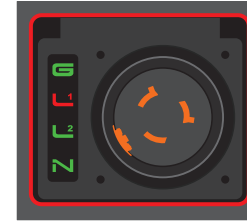
Missing Line 1 L1 - Red G, L2, N - Green Border - Flashing Red
