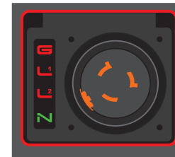
L1/L2 and Ground Reversed G, L1, L2 - Red N - Green Border - Flashing Red
