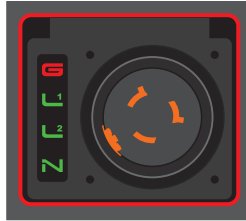
Missing Ground G - Red L1, L2, N - Green Border - Flashing Red
