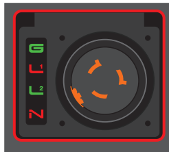
Line 1 and Neutral Reversed L1 and N - Red G, L2 - Green Border - Flashing Red
