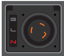
Missing Neutral N - Red G, L - Off Border - Off
