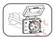
Reposition your new SafeView Power Inlet over the hole and align the screw holes. Secure the power inlet to the RV with the four screws.
